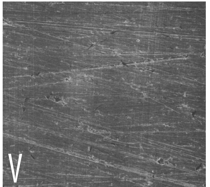
AFTER FLEX-HONE, 240 grit silicon carbide "S" photo at 1000X, "T" at 100X. More refined finish with uniform cross-hatch pattern. Surface has clean open appearance with most of torn, folded, and smeared metal removed. Excellent semi-plateaued profile. 12 to 18 \mu " (.30 to .46 \mu m) finish. Section of cylinder #A-6.
